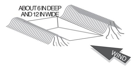
**Keyhole** - This is a modification of the Trench pit that can take advantage of a fire pit ring. The main fire is built in the fire pit, and coals for cooking are raked into the trench. Again, note that the wind enters the trench end.
